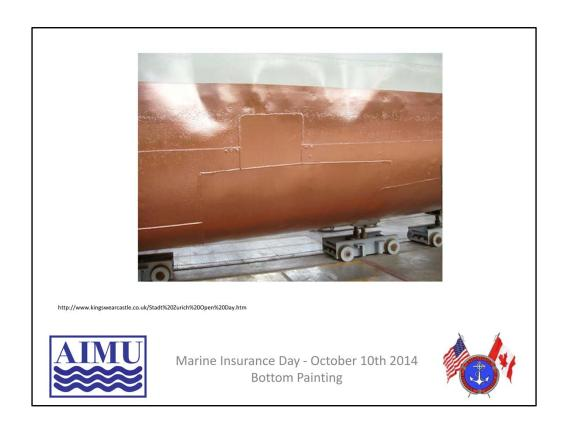
Illustration of a partial plate repair.
